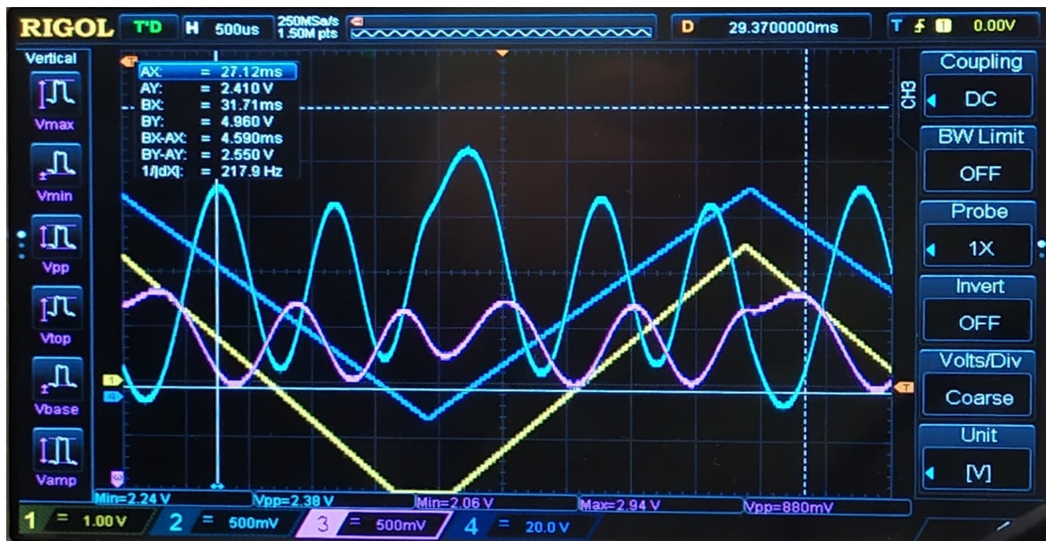
Figure 5.1: Interference signals seen on the oscilloscope. Yellow – ramp signal before the amplification, navy blue – amplified ramp signal, light blue – interference fringes for the potassium laser, purple – interference fringes for the cesium laser.
